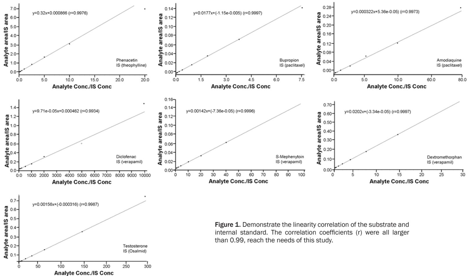
**Figure 1.** Demonstrate the linearity correlation of the substrate and internal standard. The correlation coefficients (r) were all larger than 0.99, reach the needs of this study.
