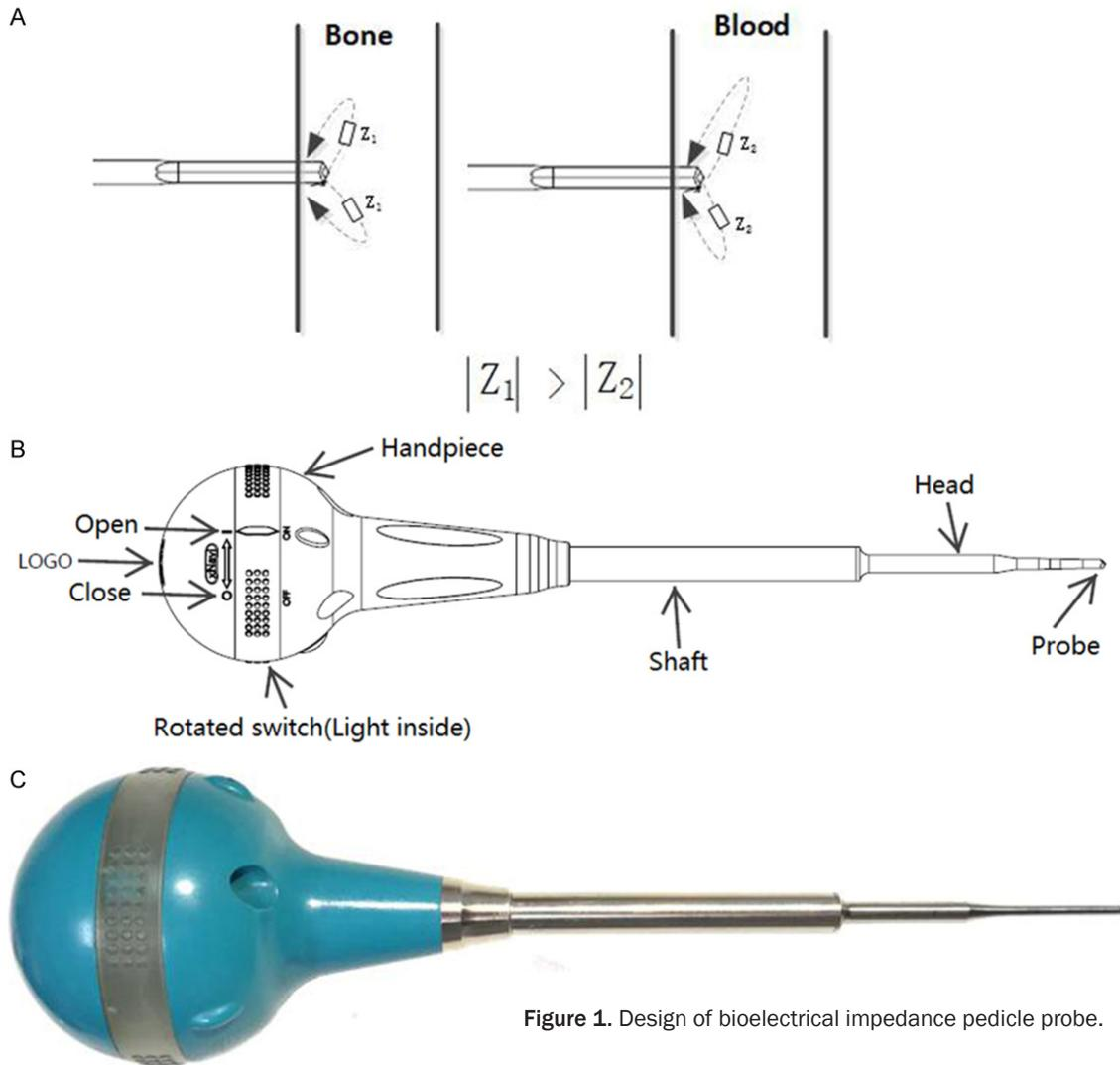
**Figure 1.** Design of bioelectrical impedance pedicle probe.
